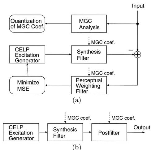
**Fig. 1** Simplified block diagram of MGC-CELP coding: (a) encoder, (b) decoder.
