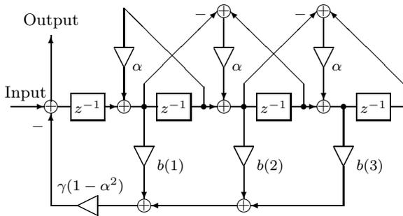
**Fig. 3** Filter structure of  $1/C(\tilde{z})$  for  $M = 3$ .
