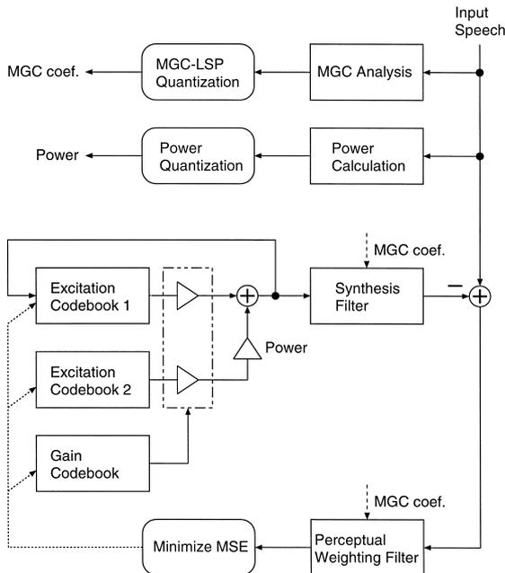
Fig. 5 Structure of wideband MGC-CELP coder at 16 kb/s.
