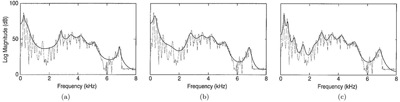
**Fig. 2** Example of spectral envelopes obtained by 20th-order analysis using a 32 ms Hamming window: (a) LP analysis, (b) MGC analysis with  $\alpha = 0$  and  $\gamma = -1/2$ , (c) MGC analysis with  $\alpha = 0.3$  and  $\gamma = -1/2$ . Thin lines represent the FFT spectrum.
